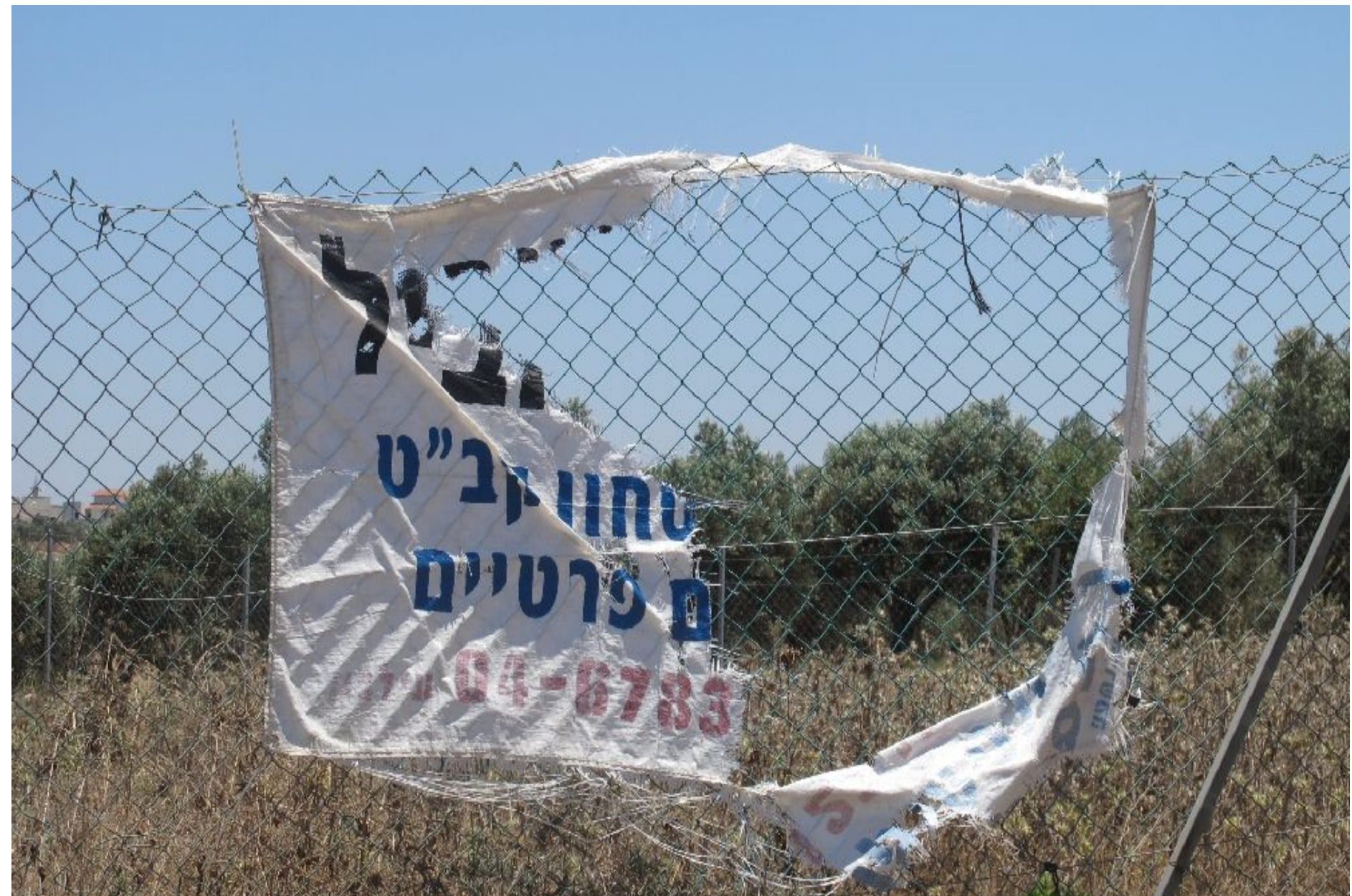
UV radiation premature degradation, picture taken on July, 6, 2012
