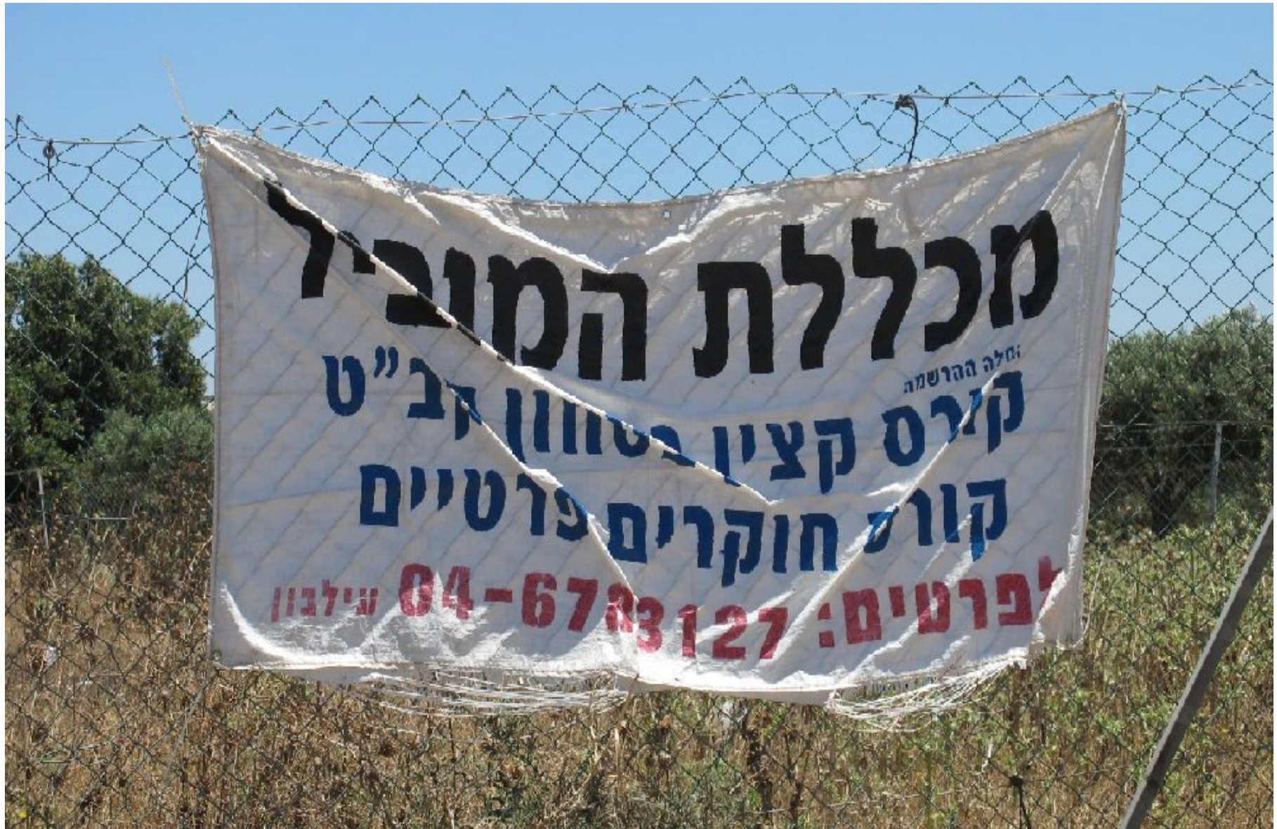
UV radiation premature degradation, picture taken on June, 8, 2012
