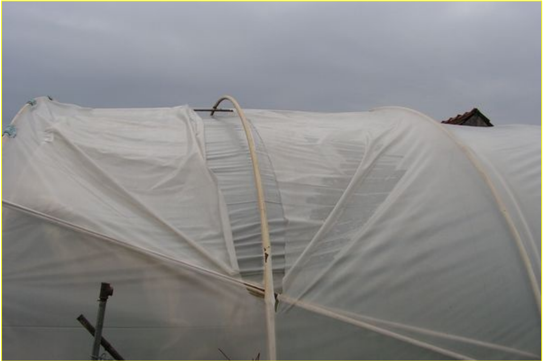
Film degradation- direct contact polyethylene and PVC
