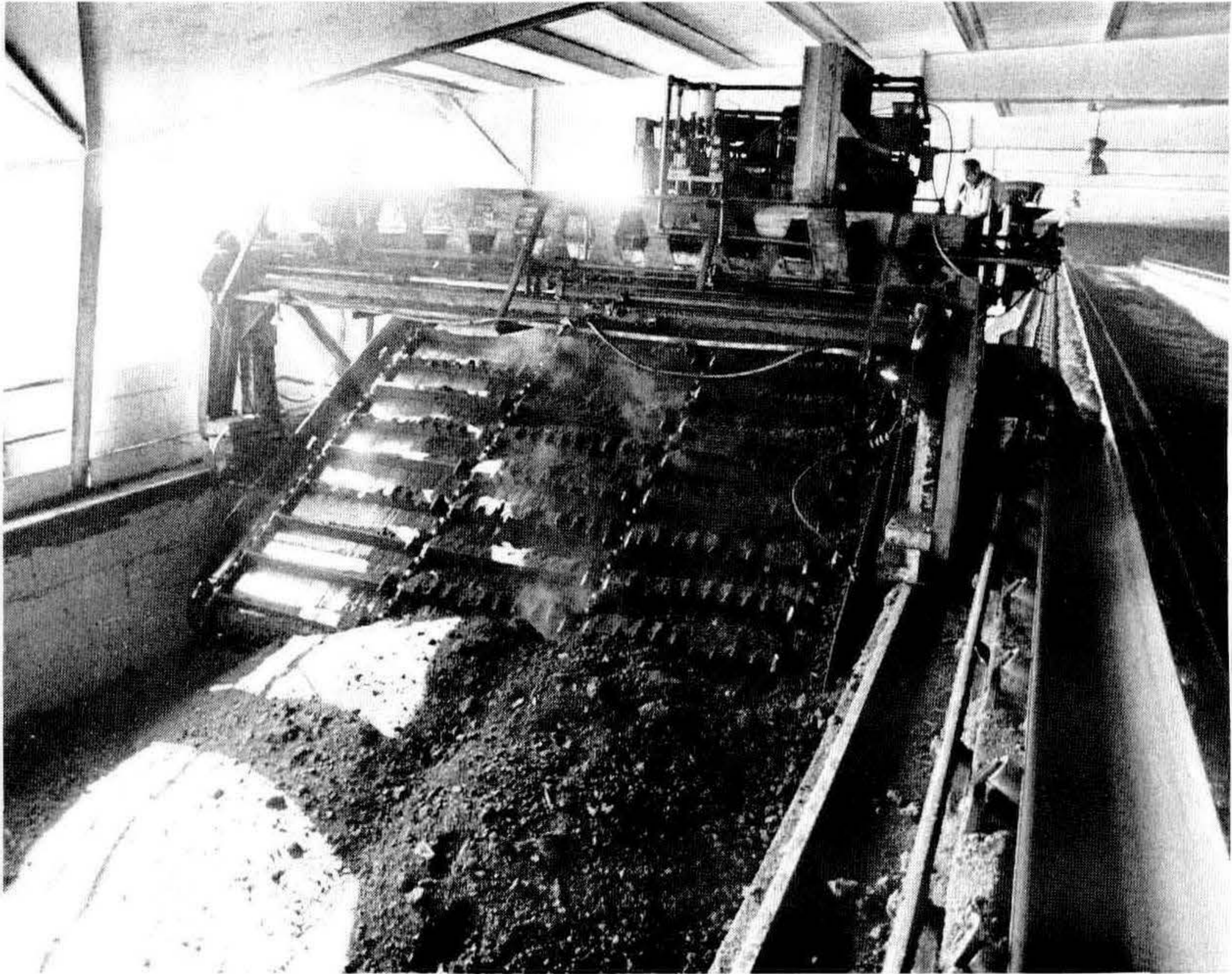
Figure 1. Compost being removed from an aerated bioreactor tank and placed onto conveyor belt. The compost is aerated by fans through perforated floors and turned frequently to expose all organic matter to thermophilic conditions. Tank ( 4 \times 7 \times 150 m) on left filled with cow manure and on right with hardwood bark.
