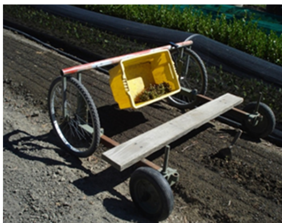
Figure 1. Tool frame with height adjustable seat.
