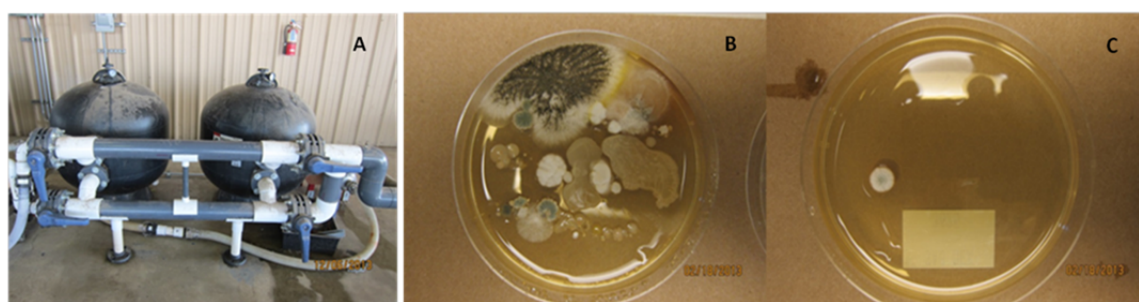
Figure 1. (A) Old pool filtering apparatus used to filter contaminants from the sanitation tanks used to clean rootstock and budwood from the field; (B) Culture plate from tank water containing fungal and bacterial contaminants prior to filtration with the old apparatus; and (C) Culture plate containing tank water contaminants after an 8-h day of filtration utilizing the old apparatus.
