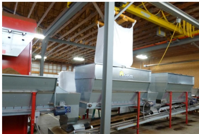
Figure 2. AgriNomix automated soil mixer.
