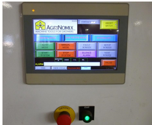
Figure 3. Touch-screen control of AgriNomix soil mixer.
