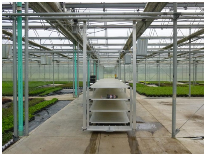
Figure 11. Powered moving cart using rail system.
