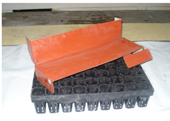
Figure 3. Plug transplanter with BCC 81 Plug Tray.
