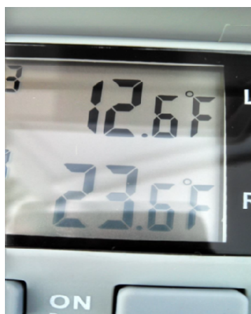
Figure 2. Comparison of outside and inside temperatures under a poly blanket.
